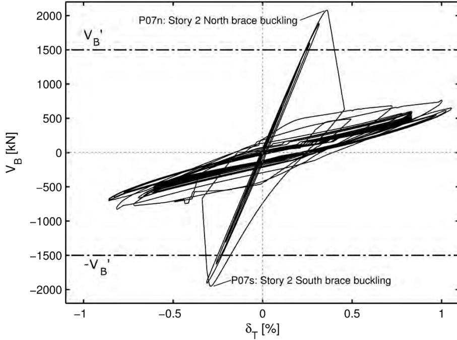
Figure 3. Base Shear vs. Total Frame Drift – Loading Pattern P (Phase I & III).
