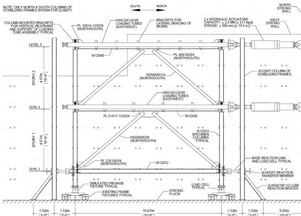
Figure 1. Experimental setup elevation.
