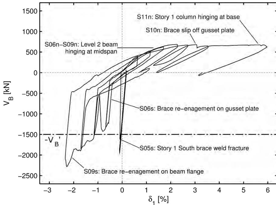
Figure 4. Base Shear vs. Story 1 Drift – Loading Pattern S (Phase IV).
